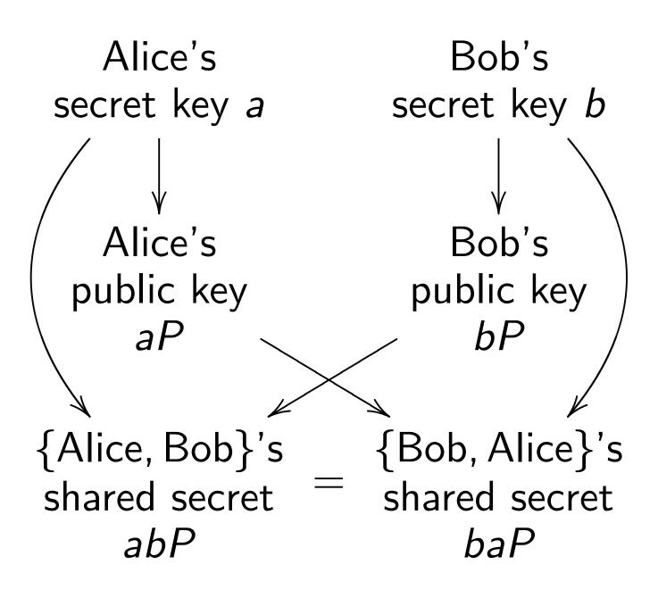
Textbook key exchange using standard point P on a standard elliptic curve E:
